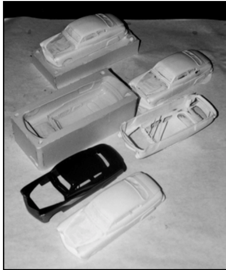
A two-piece poured block mold made of either PlatSil® 73-45 or 73-55 is ideal for most model-making or prototyping applications where thin-walled, dimensionally stable castings are required. Multiple EasyFlo™ 60 castings were made from a die-cast car model.
